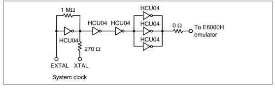
Figure 8 Clock Oscillator
